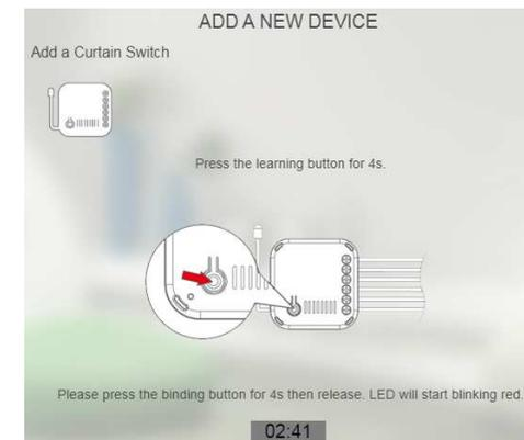
6. Press and hold the Link key for 3 seconds until its LED flashes, then release.
